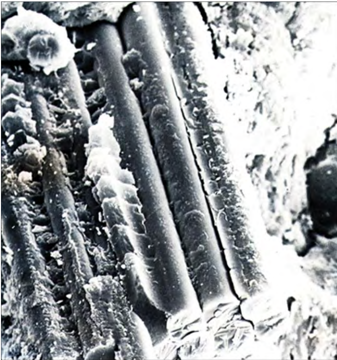
Glass fibre in aged grc-matrix magnification 1800x 12 months under water
