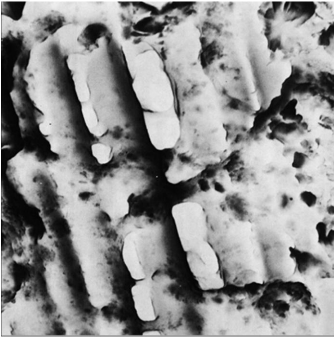
Polymer film on glass fibres magnification 1800x
