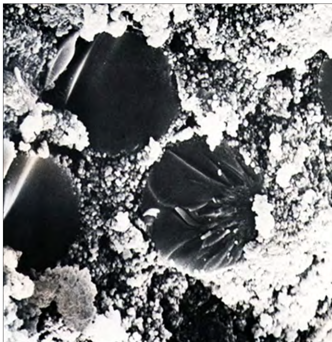
Polymer particles between magnification 5500x glass fibres
